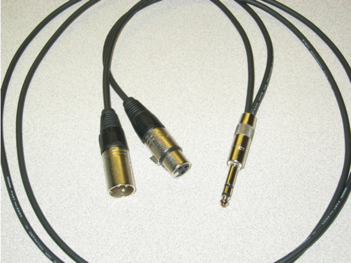
Figure 2: Finished Insert Cable
