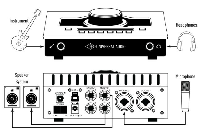
Typical Apollo Twin USB setup connections
