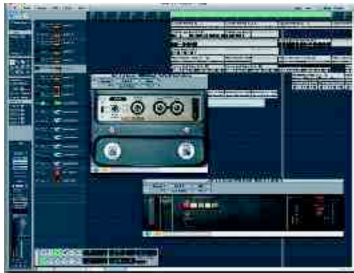
(Left) Heavy vibrato and a moderate amount of stereo chorus on an acoustic piano track, using one CE1 and one Dimension D in series.
